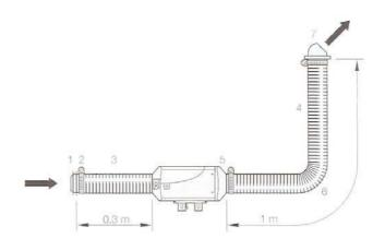
Rating sum = 5.6 and does not exceed the heater rating of 6. The installation is permissable.
